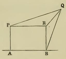
since PR is parallel to AB, which is perpendicular to the plane RBQ, PR is also perpendicular to this plane and therefore perpendicular to QR and RB. Hence PRBA is a parallelogram, and therefore AB = PR. But  $PR = PQ \cos QPR$ , since PRQ is a right angle. Therefore
